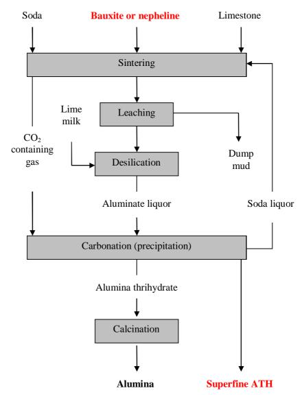
Figure 1. Flowsheet of Sinter alumina refinery.
